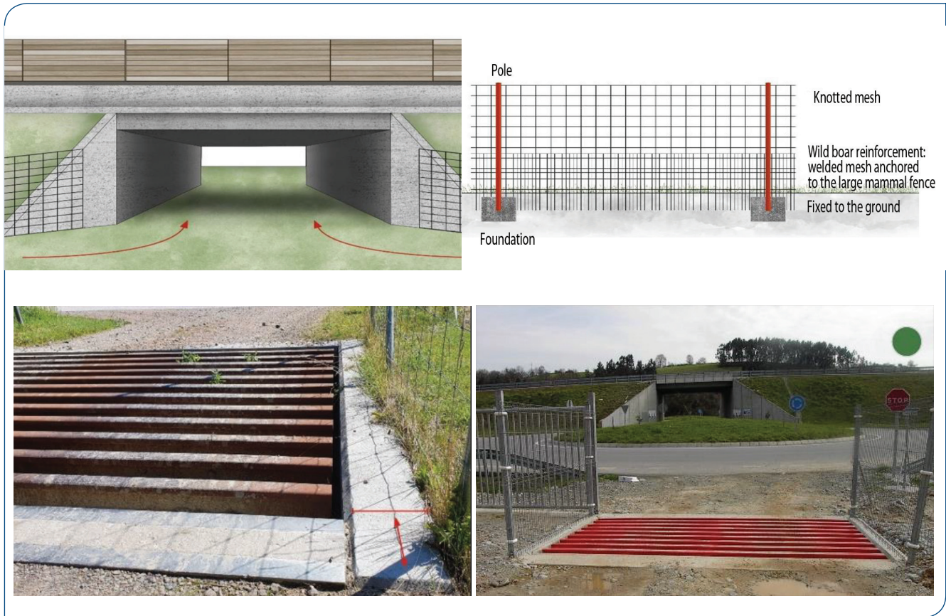
Illustration 2 - Examples of drawings providing instructions about (a) how to install fencing to guide animals to wildlife crossings, (b) how to reinforce existing fencing to avoid access of wild boar to the causeways. Red dots ('to avoid') highlight common incorrect installations, such as this example of (c) a cattle grid where the fence has been bad positioned leaving space which animals can use to bypass the grid, reducing its effectiveness. Green dots ('optimal') (d) show appropriate installation of the measure [1]
