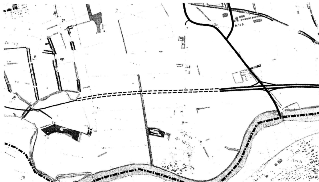
Figure 7.2 - The underground route (broken lines) of the A5 in the Grenchener Witi. (Taken from: A5 Aare to Grenchen, EIA report, Amt für Verkehr und Tiefbau, Büro für Nationalstrassen, Kanton Solothurn, October 1992).
